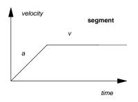
This instruction brings the system from its current position and velocity to a target position and velocity using a specified constant acceleration.
