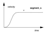
This instruction brings the system from its current position and velocity to a target position and velocity using an S curve acceleration profile.
