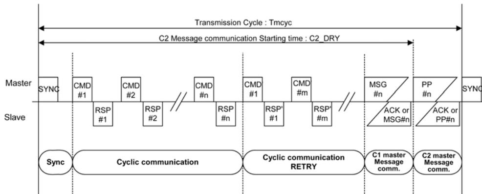
After finishing the exchange of command data and response data for all slaves, the C1 master re-sends the command data to the retry target slaves to receive the response data. After finishing the retry, the C1 master performs C1 message communication if sufficient time is available before the scheduled start of C2 (e.g., monitoring laptop computer) message communications.
